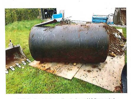
UST #1. No pinholes and/or steel or weld failures noted.
